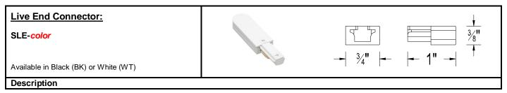
Accepts wires from transformers and connects to track. Used for live end connections when Linear Track is powered by a surface mount or remote transformer.
