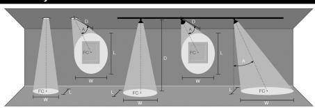
D Distance To Fixture From Wall Or Floor FC Initial Footcandle Level At Center Of Beam Beam Length (where candlepower drops to 50% of maximum)
