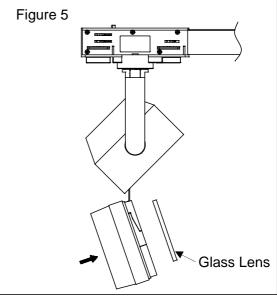
7. If necessary and beam elongating lens is not in its proper position, adjust the direction of the beam by turning the small hole on the trim around the lens until the beam is in its proper position. (See Figure 6)
