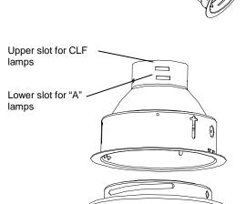
Drop lens trim twists clockwise to install
