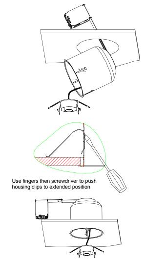
Wing springs hold and center the socket cup inside the housing.
