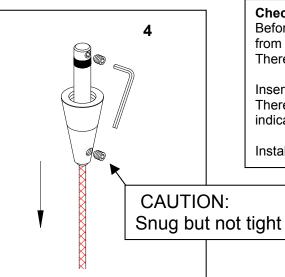
Tighten top setscrew first then lower. Smooth out any bulges in braided wire. Perform continuity check before mounting.
